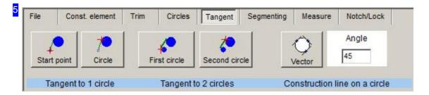
The 'Tangents on a circle' frame in the 'Tangents' tab allows you to draw a tangent to a given point on a circle. Click 'Start point' and identify the point. Click 'Circle' and identify the side of the circle to draw a tangent against.
