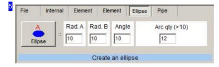
Draw ellipses in exactly the same way as other 'Contour's. Enter the required dimensions in the appropriate cells then choose 'Ellipse'.
