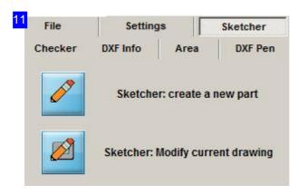
This frame allows you to open the *Sketcher* module. Click the top button to create a new part, or click the bottom button to transfer the previewed part to the *Sketcher* for editing.
