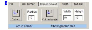
'Cut-out' allows you to make cut-outs on the internal corners of your part. Enter the required dimensions in the input cells and click the button corresponding to the cut-out you want. Use the cursor to identify the corner you want to make the cut-out at. A new frame for positioning the cursor will open to allow precision when placing your new corner.
