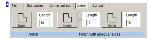
'Notch' allows you to make predefined cut-outs on your part's external corners quickly and easily. Enter the required dimensions in the input cells and choose between 'Notch' and 'Notch with 2 different sides'. A new frame for positioning the cursor will open to allow precision when placing your new corner.
