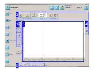
This is the *Sketcher* screen. The centre area [3] is an open drawing space with a workspace and status bar. The workspace can be a given area (pre-cut), an external contour or a restricted are in the classical sense.
