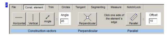
The 'Const. Elem' tab offers options for creating construction lines. If you set a separate line color for construction lines you will be able to work on (check, edit, delete) them more quickly and accurately.
