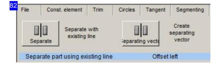
A separating vector can also be placed directly onto an existing line, e.g. an open contour. This separates the part, and moves the separated part left. You should always use this function moving through parts from left to right. Insure that the separating line ends at a contour so that the contour can be closed at the line afterwards.
