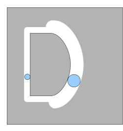
Certain machines such as stamping or beveling tools require you to use different-sized tools in order to allow free clearance space for the next tool to do its work. These free spaces may overlap each other, but may not cross into the actual workpiece.
