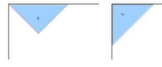
Here we see that even the first part must be nested onto the sheet, despite not having to fit in with any other parts. The most efficient use of material is illustrated by the example on the right hand side.
