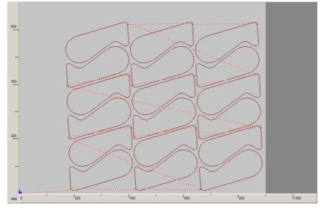
When nesting manually, you can stretch a box to show an area into which to duplicate areas which are already populated. The positioning of the original parts has a defining influence on the effectiveness of the nest. As shown below, when the first parts are set out well, an efficient nest can be created.
