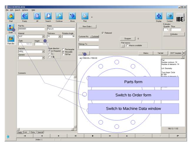
Enter all part data in the relevant field, remembering to confirm your entries by clicking the "return" button. The part will automatically be allocated a new part number.
