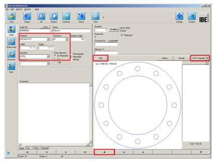
Select: [homepage] [orders] [order][+]. Select a template and allocate the order to a machine. Select the material and its thickness.
