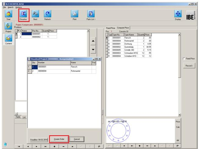
Click [dissolve] to open a dialog box for entering the quantity of parts, a further dialog box will appear with a list of the individual cut parts. To transfer the parts to orders, select [create orders]. The production deadline is shown at the bottom-left. To change this deadline, click the button and select from a calender.
