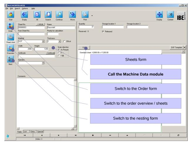
Enter all sheet data into the relevant fields of this form and confirm your entries with the "Return" button. Switch to the Machine Data module <sup>20</sup> to change a drawing's geometric properties as required.
