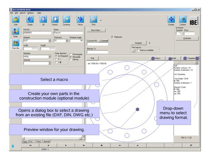
The selected/created part is displayed in the preview window. Faulty DXF files can be checked using the DXF-Checker, which will fix any errors for you.
