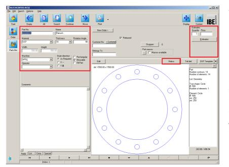
To enter a new part, select: [homepage] [orders] [parts bin] [+]. Enter a part name and select the material, thickness and machine. Select [macro] and develop your part from the macro template.
