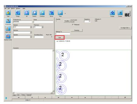
Select: [homepage] [processing plans] Select the required plan from the list and click [edit] to move on to the machine data screen and generate your NC code.
